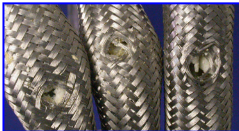
Water Heater Connectors- Puncture Damage
