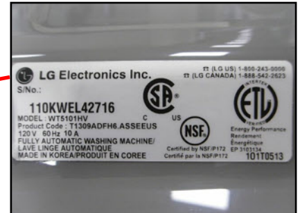
Location of the rating label with model and serial number on the washer
