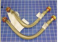
DPI still receives many failed Watts water heater connectors each year. These connectors can be easily identified by their product tags marked WATTS® (top left) or by the Watts "W" logo marking on the crimp sleeve (bottom left). Though they were mostly produced in the mid-2000s, thousands of these lines are likely still in service.
